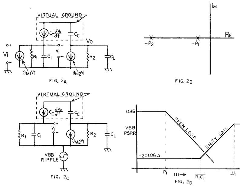
Fig. 2. (a) The new frequency compensation concept. (b) Resultant pole locations in  $s$ -plane. (c) Small signal model for  $V_{BB}$  PSRR analysis. (d) Expected  $V_{BB}$  PSRR frequency response of Fig. 1(a).
