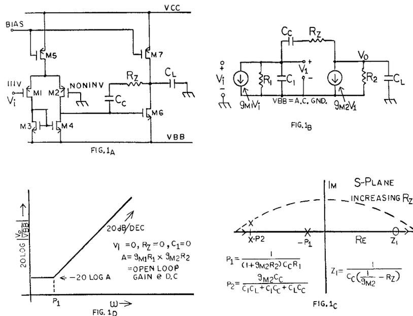
Fig. 1. (a) Commonly used two-stage operational amplifier. (b) Small signal equivalent model for the two-stage amplifier. (c) Pole-zero diagram of Fig. 1(b). (d)  $V_{BB}$  PSRR in unity gain configuration.
