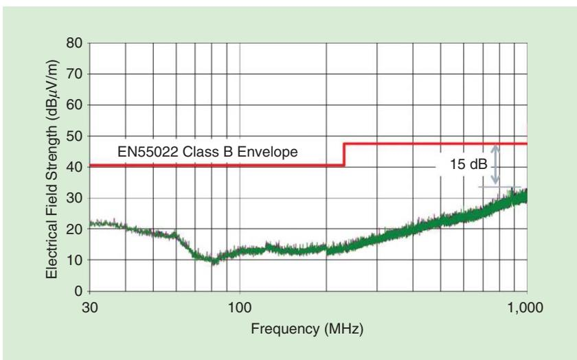
FIGURE 30: Measured radiated emission.
