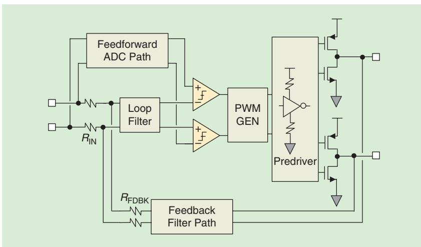
FIGURE 23: The enhanced class D architecture.
