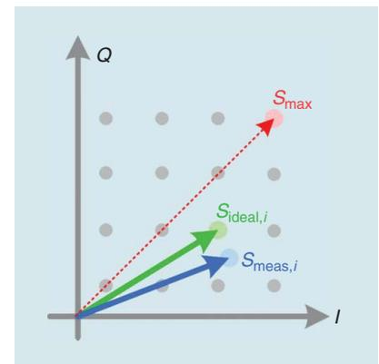
**FIGURE 1:** A normalized constellation diagram for 64-QAM. Only the first quadrant is shown for simplicity.
