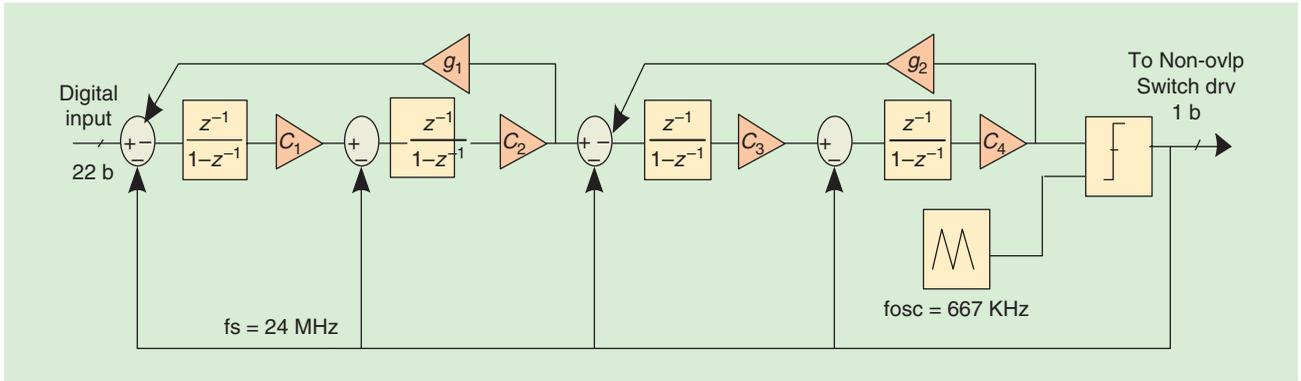
FIGURE 14: A digital PWM modulator.
