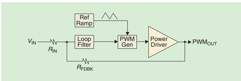
FIGURE 16: Conventional analog feedback class D architecture.
