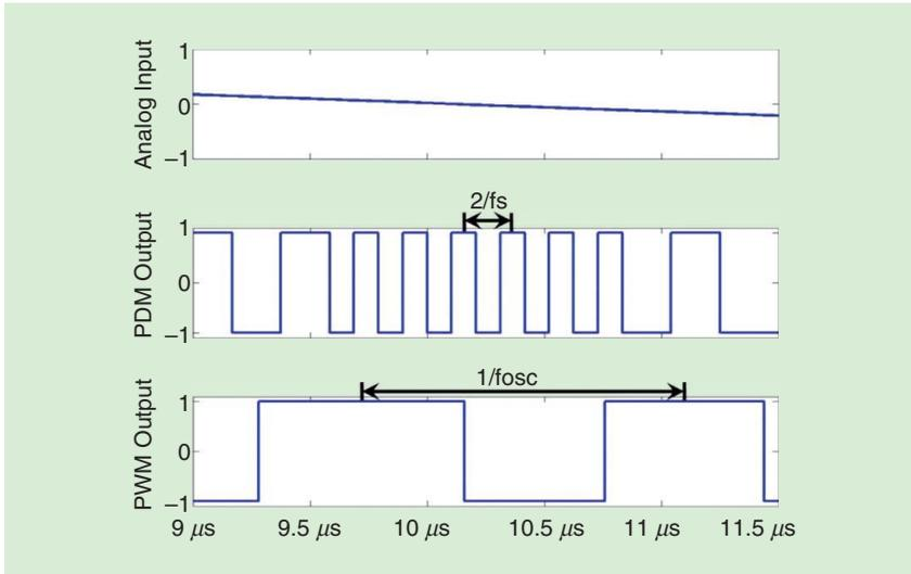
FIGURE 10: A comparison of PDM and PWM waveforms.
