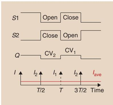
**FIGURE 3:** The states of S1 and S2, the amount of charge on the capacitor, and the current from  $V_1$  to capacitor ( $I_1$ ) and from capacitor to  $V_2$  ( $I_2$ ) as functions of time.
