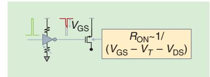
FIGURE 20: Switch-on resistance control.
