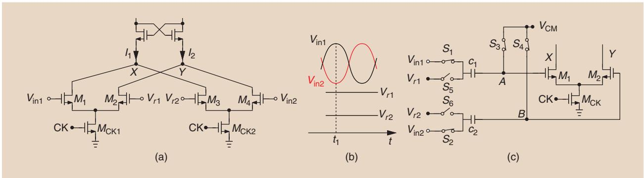
**FIGURE 4:** (a) A comparator input stage based on two differential pairs, (b) the effect of different CM levels, and (c) an alternative input stage.
