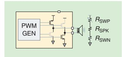
FIGURE 19: Programmable driver strength.
