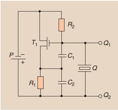
**FIGURE 8:** The MOS crystal oscillators patented by Luscher.
