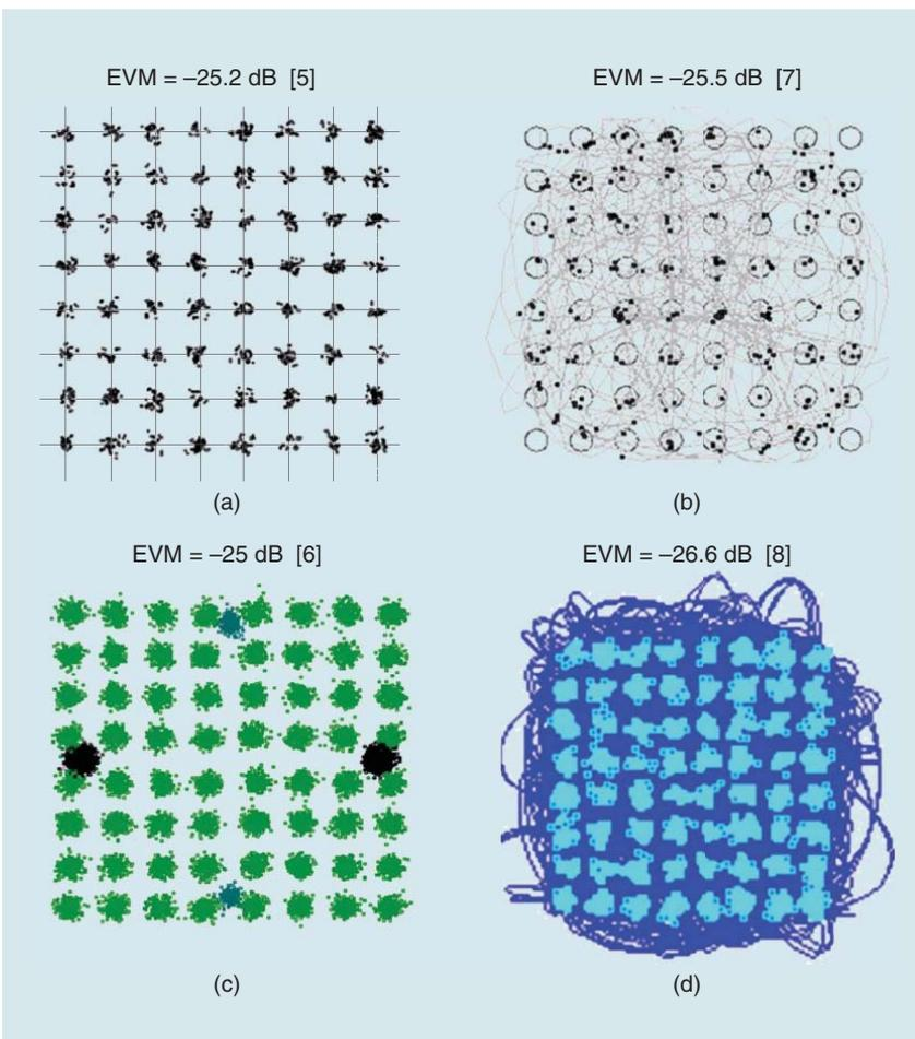
**FIGURE 2:** Measured constellation and reported EVM of four state-of-the-art mm-wave PAs for future 5G presented at the IEEE International Solid-State Circuits Conference in recent years [5]–[8]. Note that (b) has no points at the constellation corners, clearly showing circuit compression, which is not seen in the other measurements (yet the same EVM value is reported).
