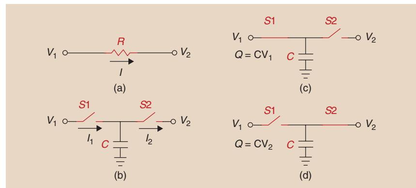
FIGURE 2: (a) A simple resistor, (b) a capacitor and two switches that act like a resistor, (c) the switched-capacitor circuit when  $S_1$  is closed and  $S_2$  is open, and (d) the switched-capacitor circuit when  $S_1$  is open and  $S_2$  is closed.
