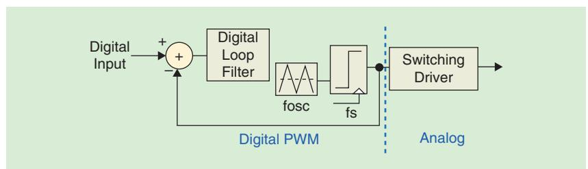
FIGURE 13: A digital PWM class D amplifier.
