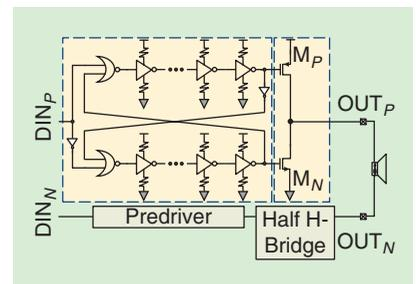
FIGURE 17: Edge rate control for EMI reduction.
