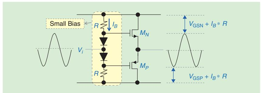
FIGURE 3: A CMOS class AB audio amplifier.
