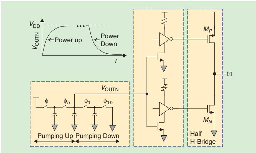
FIGURE 21: Class D power driver ramping.
