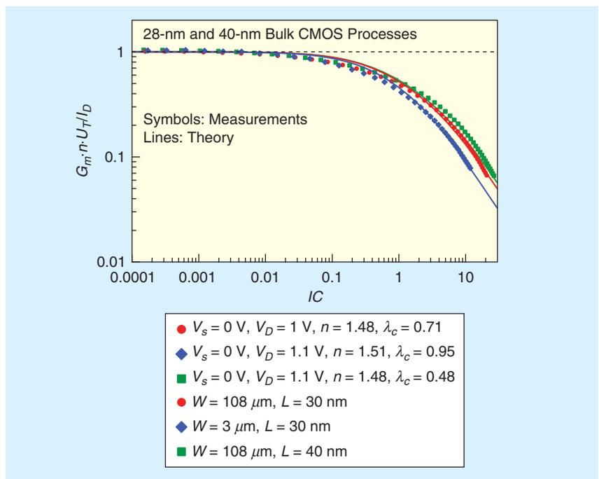
**FIGURE 8:** Normalized transconductance efficiency  $g_{ms}/IC$  versus  $IC$  measured on minimum length transistors from a 40-nm and two different 28-nm bulk CMOS processes.
