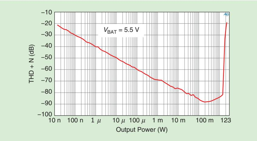
FIGURE 27: Measured THD+N versus output power.
