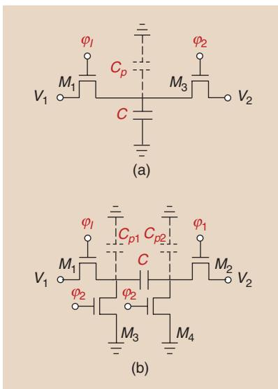
**FIGURE 4:** (a) A straightforward implementation of a switched-capacitor circuit implementing a resistor using NMOS transistors and (b) a parasitic-insensitive switched-capacitor circuit implementing a resistor.
