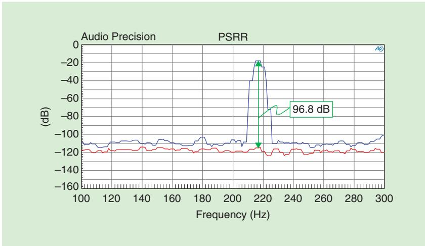
FIGURE 28: Measured PSRR.
