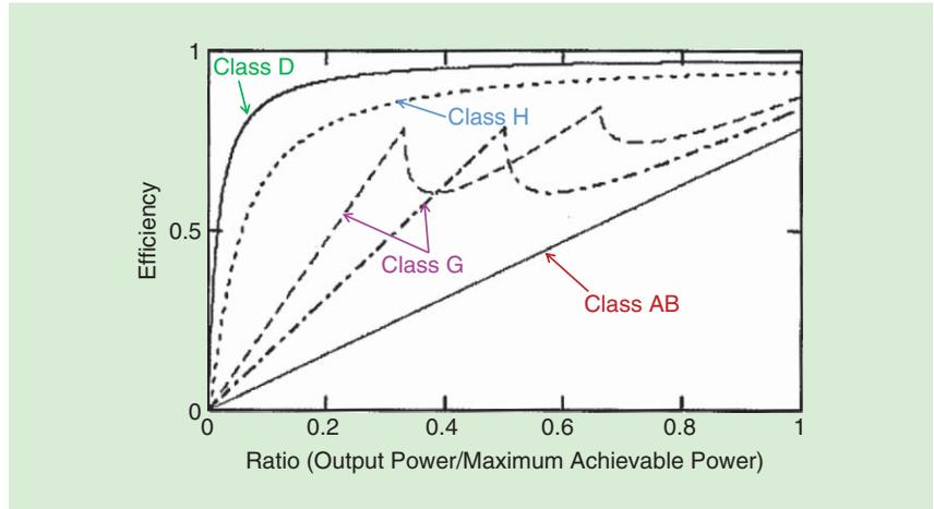
FIGURE 7: An efficiency comparison.
