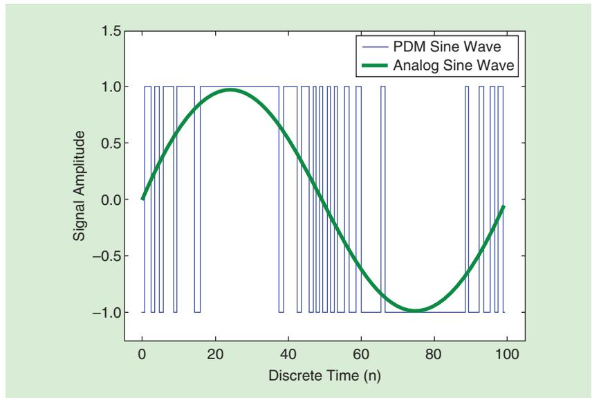
FIGURE 8: A PDM waveform.
