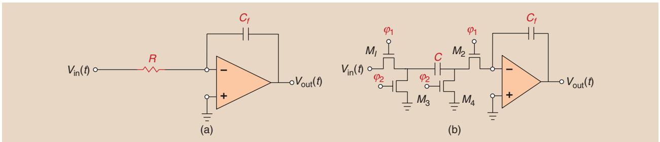
FIGURE 5: (a) An integrator using a resistor and a capacitor and (b) an integrator replacing the resistor with a parasitic-insensitive switched capacitor.
