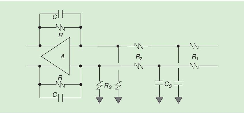
FIGURE 25: A feedback filter path.
