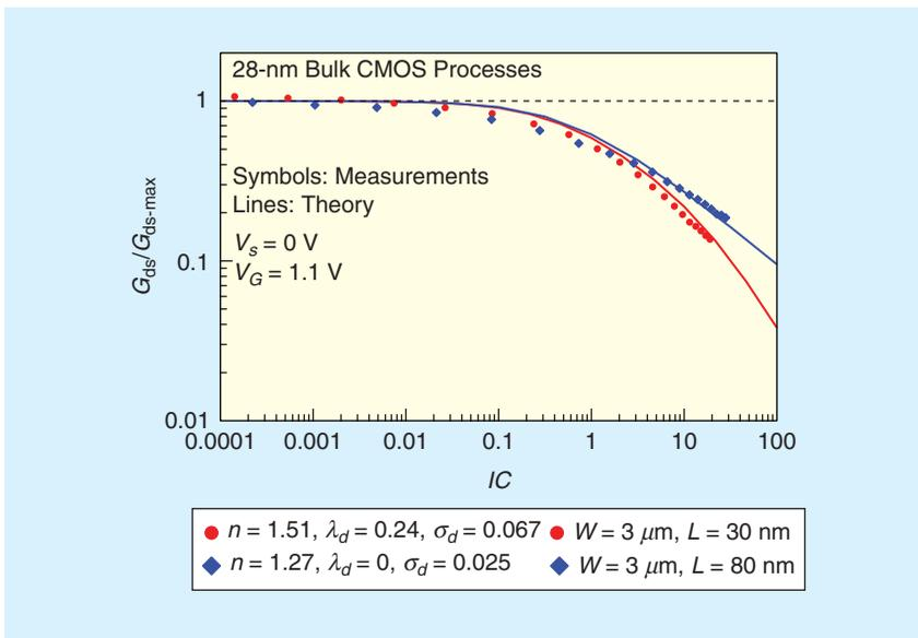
**FIGURE 9:** Output conductance-to-current ratio  $G_{ds}/G_{ds-max}$  versus  $IC$  measured on minimum and medium length transistors from a 28-nm bulk CMOS process.
