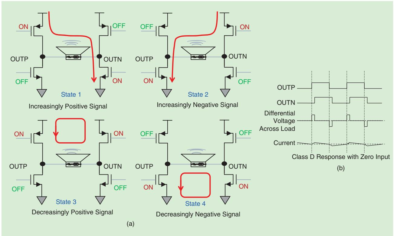
FIGURE 12: (a) A BD/filterless modulation scheme and (b) BD/filterless waveforms.
