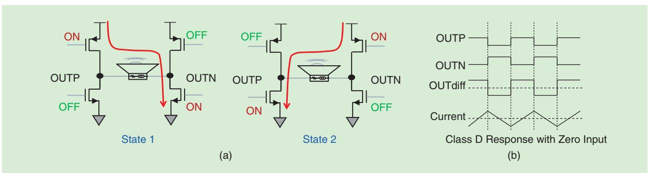
FIGURE 11: (a) An AD modulation scheme and (b) AD modulation waveforms.
