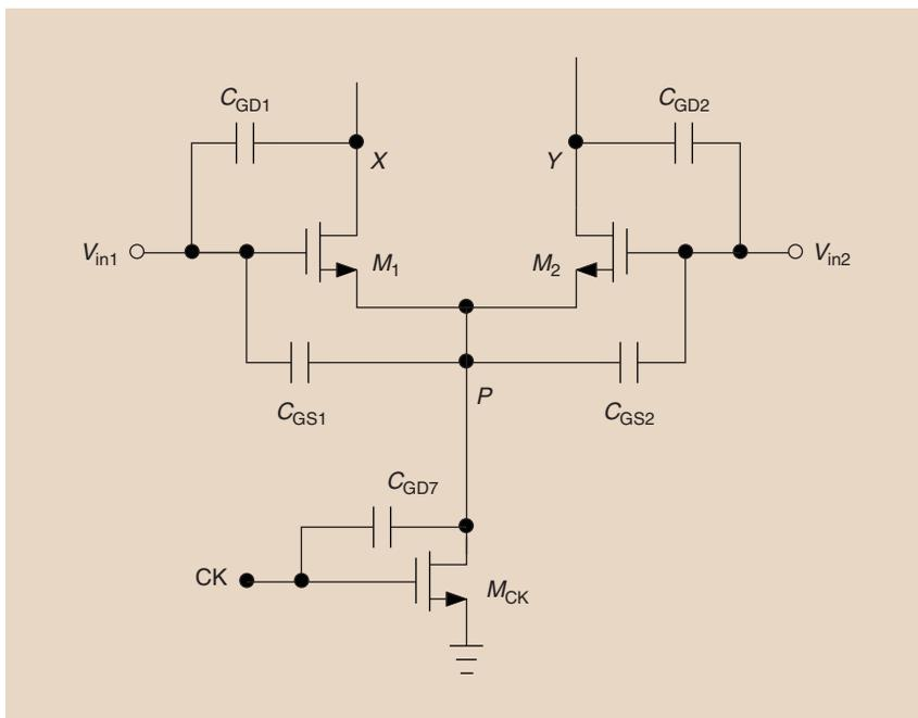
FIGURE 2: The input stage of a StrongArm latch.
