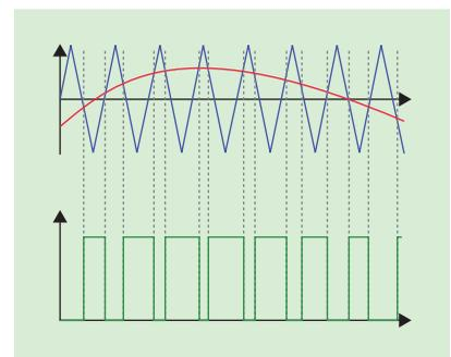
FIGURE 9: A PWM waveform.
