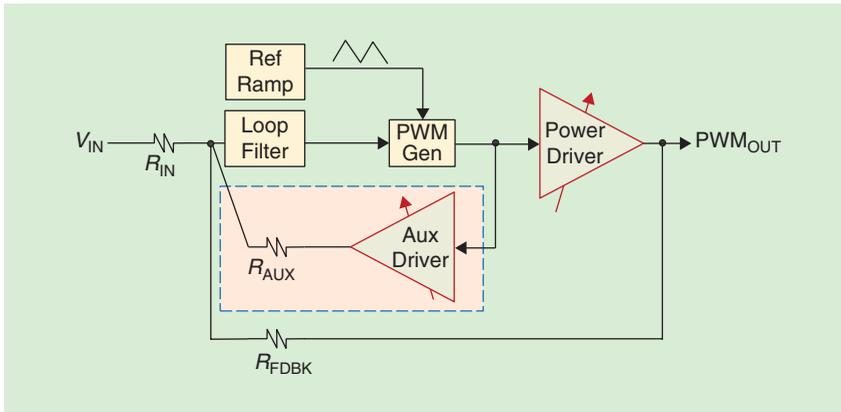
FIGURE 18: A class D amplifier with an auxiliary loop.
