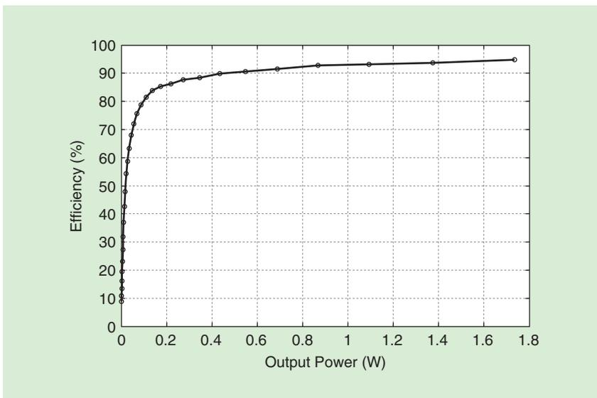
FIGURE 29: Measured class D efficiency.
