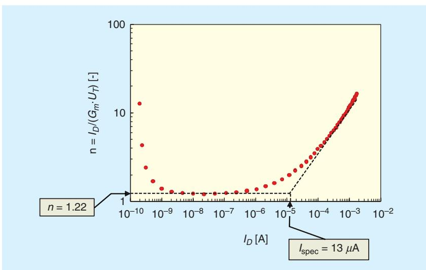
**FIGURE 10:** The extraction of the slope factor  $n$  and the specific current  $I_{spec}$ .
