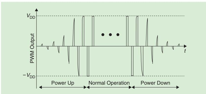
FIGURE 22: The differential PWM pulses during power up and power down.
